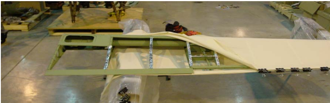
Figure 3: Placement of cotton bag over aileron
