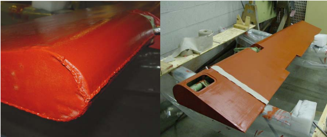
Figures 5 and 6: Well saturated doped fabric surface and the application of rib strips
