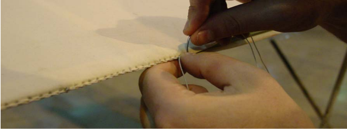
Figure 4: Stitching of trailing edge seam
