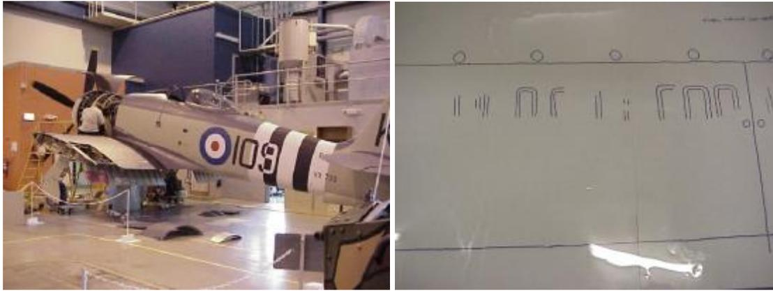
**Figs 3a and 3b:** The original paint on the Memorial’s Hawker Sea Fury FB.11 Fighter Bomber was retained under new paint which recreated its appearance when it was still in service. In a shaft of raking light one day, rocket markings in the original paint on the outside of the cockpit became visible as proud areas under the new paint. These confirmed the aircraft’s service history, which before had been in some doubt.
