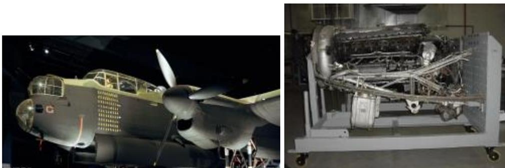
**Figs 4a and 4b:** Initial plans for the restoration of the Lancaster Bomber “G for George” included \$30,000 for the engines to be overhauled by Rolls Royce engineers. At an energetic round-table discussion however, we realised that we weren’t intending to operate the engines, full dismantling would remove all evidence of WW2 assembly and maintenance practices, and what we had initially thought was corrosion in the
