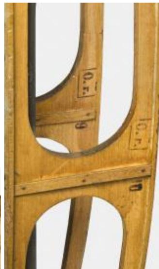
**Figs 2a and 2b:** The wooden wings of the Memorial’s Albatros D.Va fighter aircraft provide information not only on the early use of aircraft in war, but also on the materials, construction and repair techniques in use at the time (note the bound and glued repair in 2a), the beginnings of mass production (note the rib numbering system in 2b), and even a connection to the individual people who made the aircraft (note the signed certification panel in 2a).
